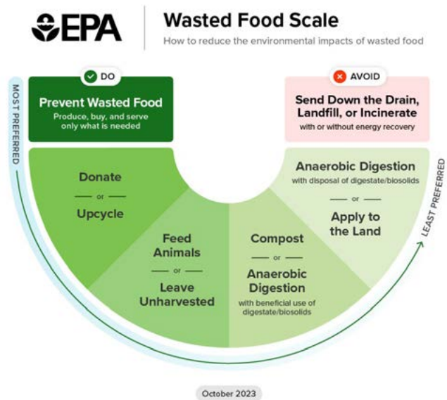
Figure 6.11 The wasted food scale: EPA’s new ranking of wasted food pathways based on lifecycle assessment and circularity assessment
