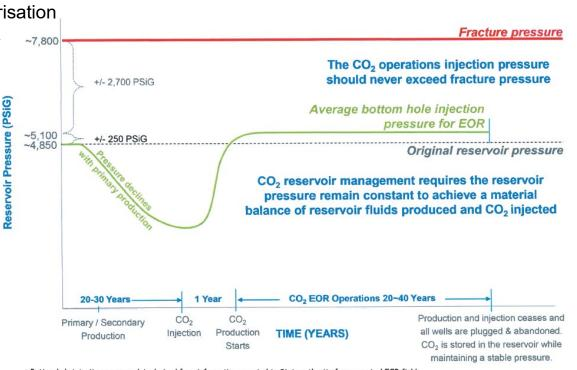
\* Bottom hole injection pressure data derived from information reported to State authority from an actual EOR field \* Fracture pressure is the amount of pressure required to permanently deform the rock structure of the formation
