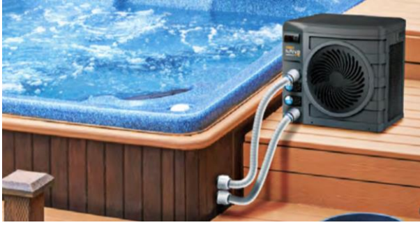
Figure 29. Example of a plug'n play compact pool heat pump with a capacity on 2,3 - 2,9 kW (at T_{air} 15 - 26°C and T_{water} 26°C) for small swimming pools up to 20 m 3 or spas. It's corresponding COP is 3,9 – 5 and it measures 385 x 400 x 280 mm 342 .
