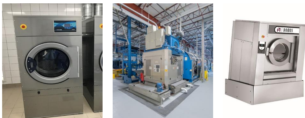
Figure 4. (From left-to-right) dryer 21 , tunnel-washer 22 , big washer-extractor 23
