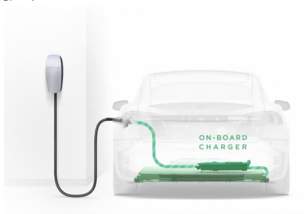
Figure 92: Illustration of the on-board charger
